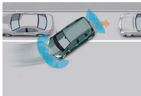
Parking: Active parking assist steers the car into the parking space, while the driver merely accelerates and brakes.
